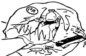
GLOVE-BAG for work with air sensitive materials
