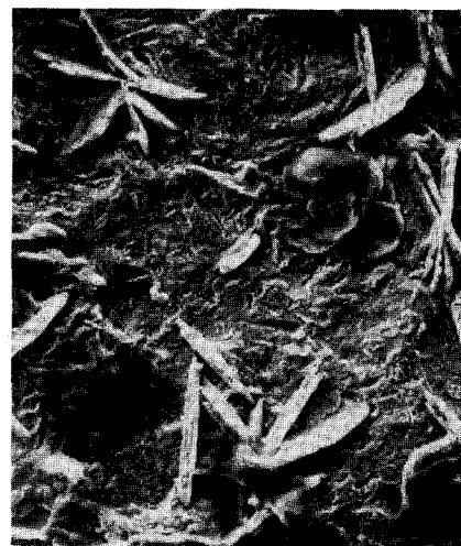
Fig. 1. Elemental X-ray analysis (above) and micrograph (right) of phosphate coating on alloy steel at 500x.
