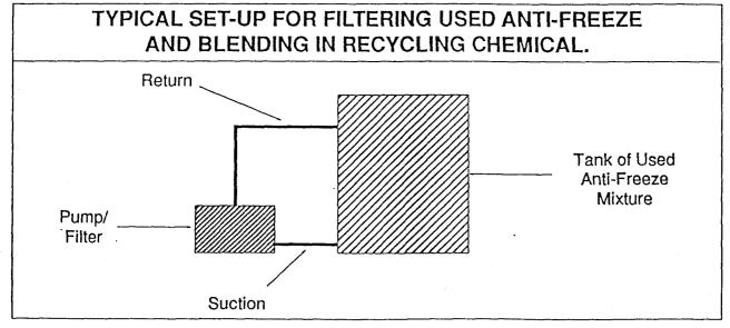
The tank, as mentioned earlier, should be sized to suit the needs of the fleet in question. Steel is certainly an acceptable material, but a plastic, such as polyethylene, is also good.
