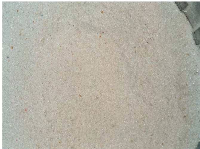
Fig 1: Photograph of crushed white glass cullet.
