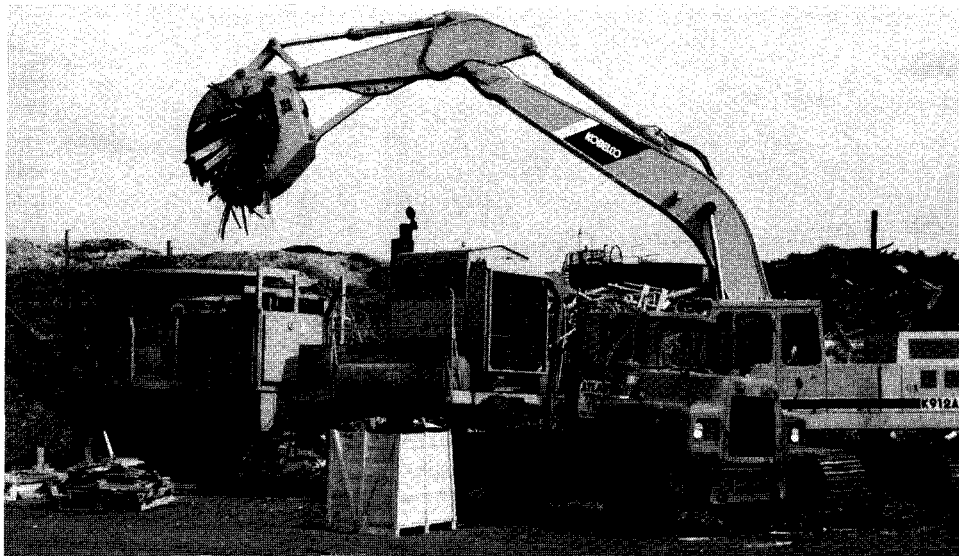
An excavator with a grapple arm loads construction wood debris into a tub grinder at Advanced Enterprises Recycling's site.
