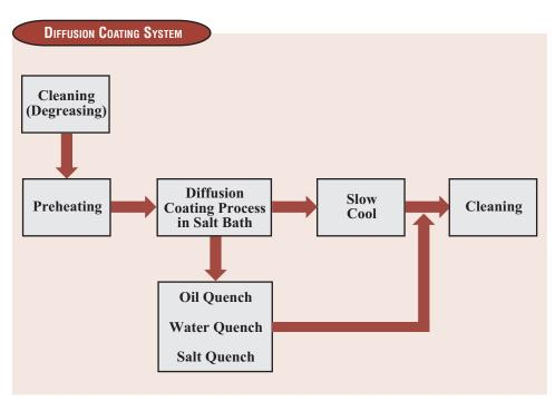
The unique coating process is based on thermal diffusion technology which forms a VC layer on the surface of steel and stainless steel base materials. Tool and die manufacturers could reduce energy use by 35% to 50%.
