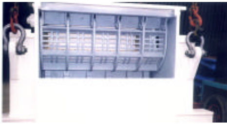
Figure 2b Mono Shear Front Grid
