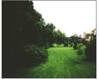
**Description**: Grassed filter strips (a.k.a., vegetated filter strips, filter strips, and grassed filters) are vegetated surfaces that are designed to treat sheet flow from adjacent surfaces and remove pollutants through filtration and infiltration.
