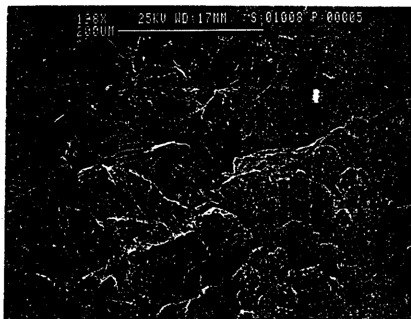
Figure 7. Unpolished sample for 1008 at open air and 1000°C with \text{FeS} : \text{Na}_2\text{S} = 82 : 18 sample ( above ), flake ( below )
