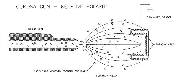
THE LACK OF POWDER IN THE FARADAY AREAS IS CAUSED BY REPULSION OF SIMILARLY CHARGED POWDER PARTICLES AND AIR POCKETS IN CORNERS OF THE PRODUCT.
