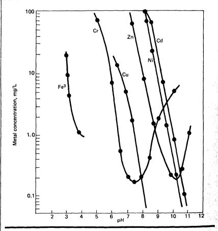
Precipitation of heavy metals as hydroxides
