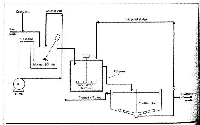
Typical continuous-treatment system for heavy metals
