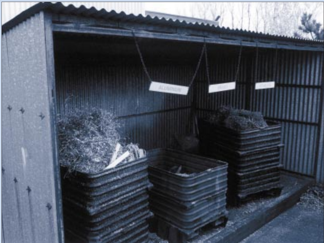
Covered and bunded swarf storage area at Kidde Graviner
