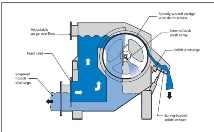
Fig 6 Typical rotary drum screen
