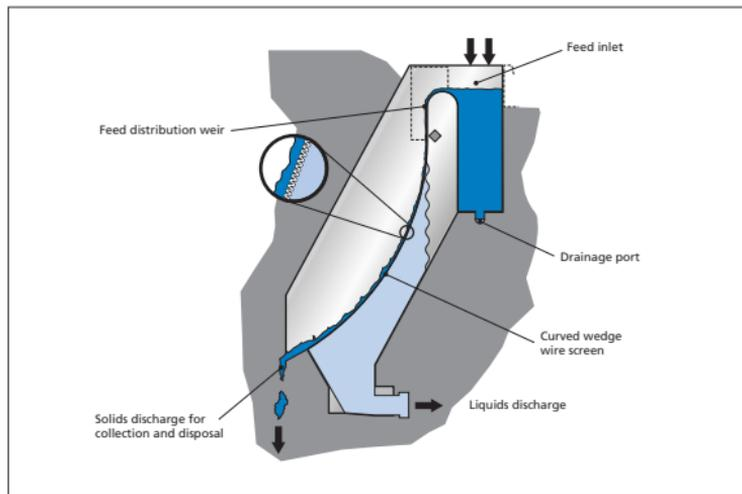
Fig 4 Typical static wedge screen
