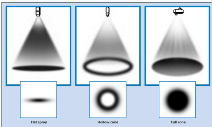
Fig 3 Spray nozzles suitable for use in poultry processing and their spray patterns
