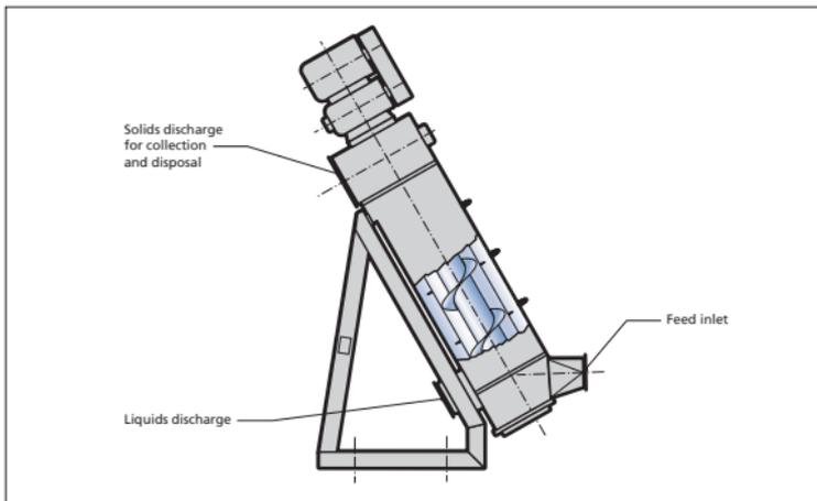
Fig 5 Typical inclined screw press
