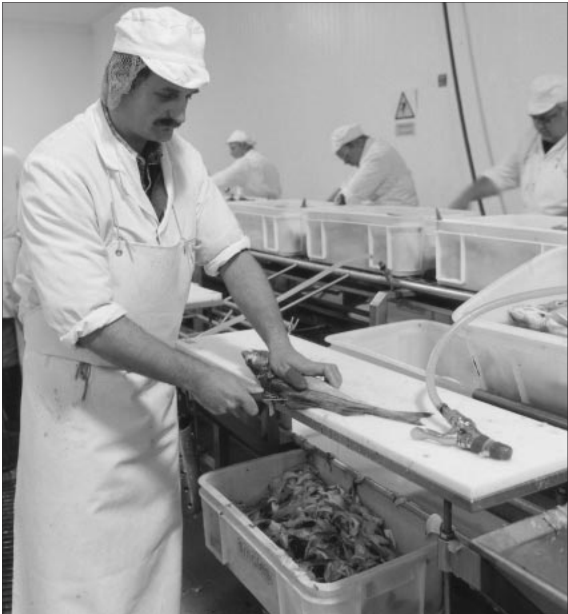
Catch basket to collect waste falling off the bench
