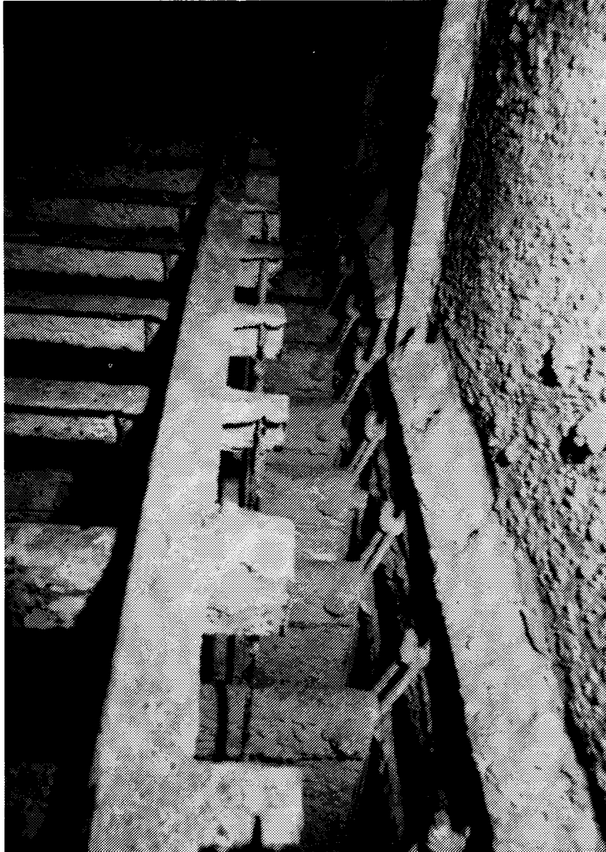
Figure 6-13. Upper baffle used as plate suspension.
