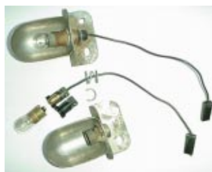
Example of a GM hood light switch. Photo Credit: Tom Corbett, NY Department of Environmental Conservation
