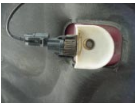
Example of a DaimlerChrysler hood light switch. Photo Credit: Tom Corbett, NY Department of Environmental Conservation
