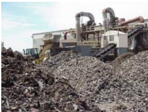
Loading of non-ferrous and heavy ASR into separation plant at Huron Valley Steel Corporation, Belleville, MI. Photo Credit: Huron Valley Steel Corporation.
