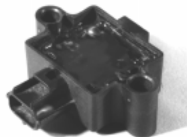
ABS Acceleration Sensor from a 1999 Jeep Grand Cherokee. Photo Credit: Jeff Gearhart.
