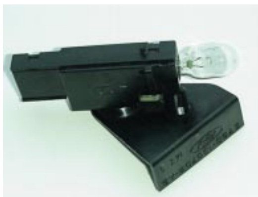
Example of a Ford truck light switch. Photo Credit: Tom Corbett, NY Department of Environmental Conservation
