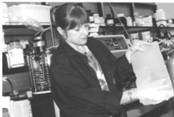
Sandia National Laboratories technologist Patti Sawyer holds a sheet of the unheated epoxy adhesive. In the unheated state, it looks and feels like a rubber band.
