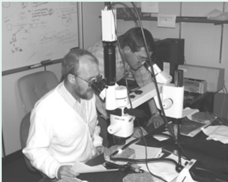
Kansas City Plant engineers Steve Cave (left) and Chris Baumgart examine concrete samples using the R&D 100 Award-winning automated electronic imaging process they co-developed. The process scans concrete and calculates 16 microscopical properties with precision to one-half micron.
