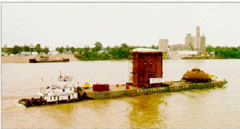
The vessel, head, internal items, and transport equipment, weighing a total of 2,200 tons, were loaded onto a 276-foot barge and shipped 750 miles up the Ohio River. After departing Mt. Vernon (bottom), the loaded barge passed under 49 bridges, including those at Cincinnati (top).
