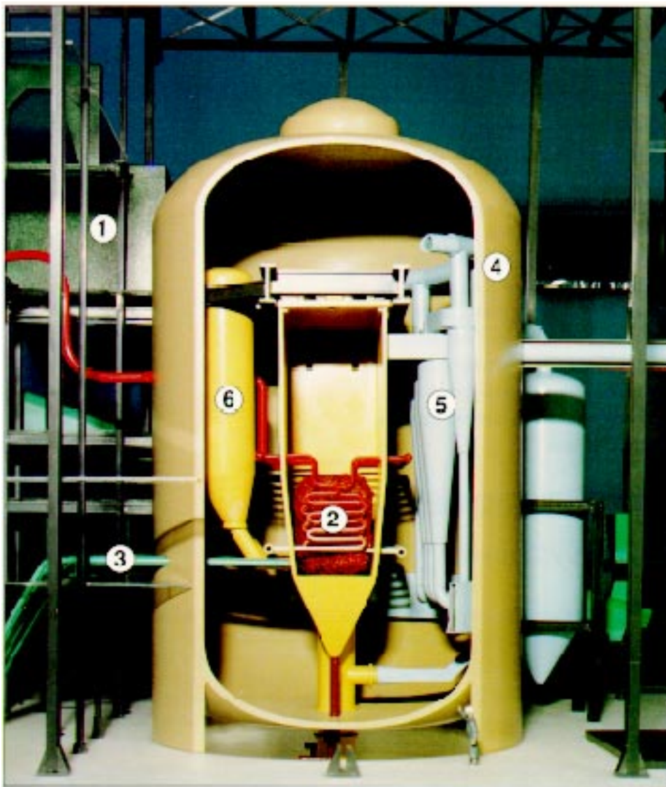
This scale model of Tidd's pressure vessel shows (1) the dolomite feed system, (2) boiler tubes suspended in the fluidized bed, (3) coal feed lines, (4) vessel wall, (5) two-stage cyclone train, and (6) bed ash reinjection vessel.
