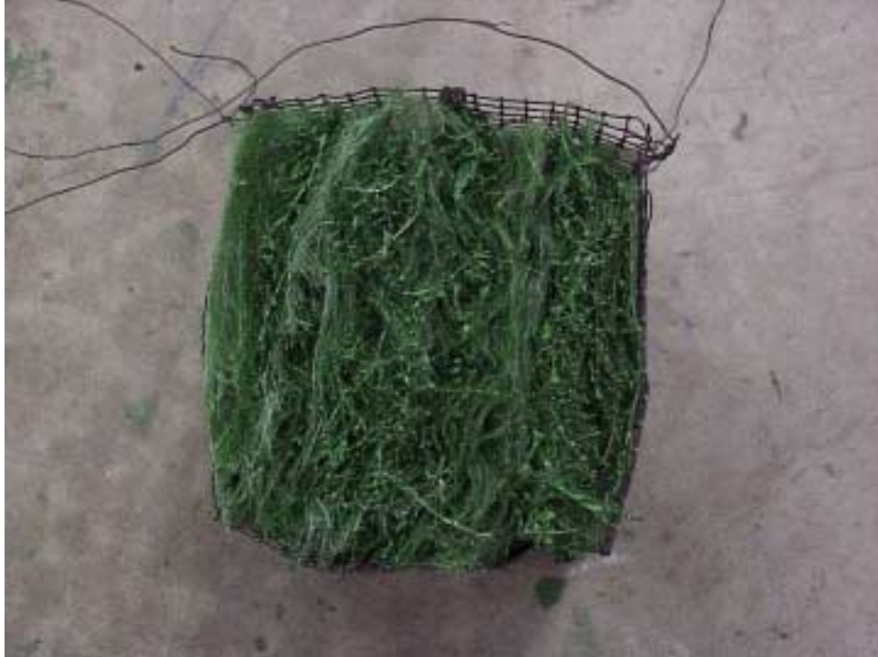
Figure 9 - Paint loaded filters in wire mesh before test.
