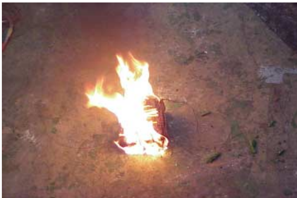
Figure 13 - Increased air velocity to the center induced flaming ignition.
