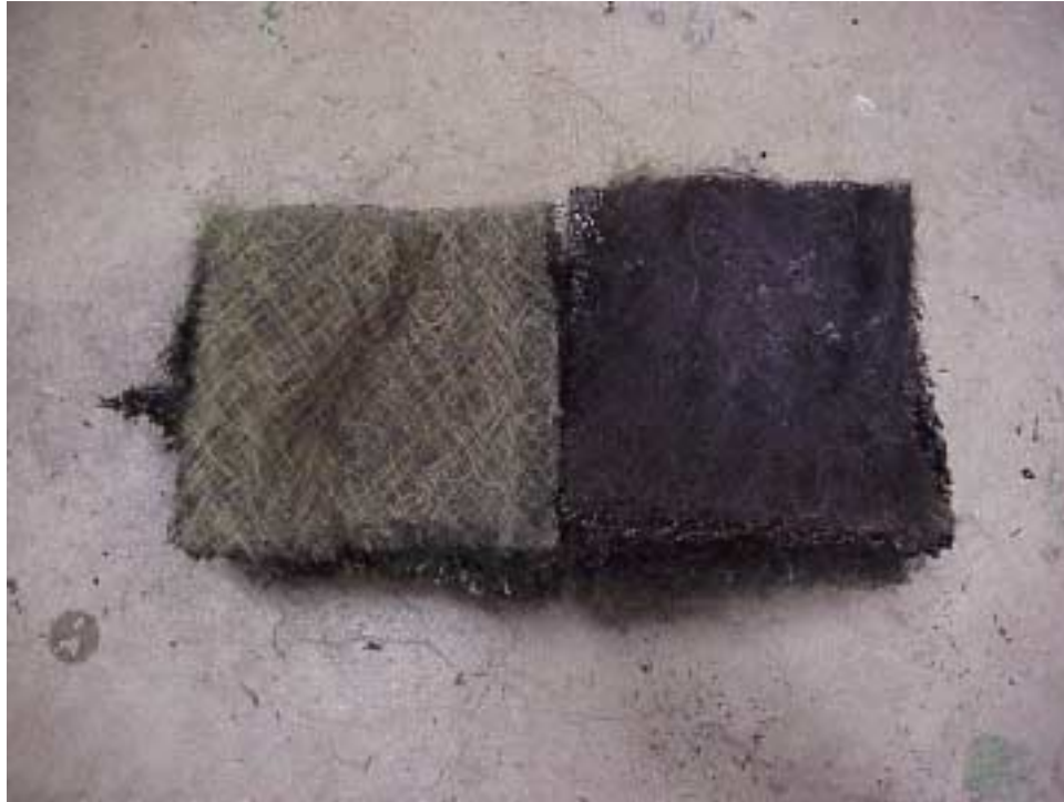
Figure 10 - Paint loaded filter after test (sub-critical).
