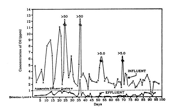
Figure 1. Influent and Effluent Concentrations (from Electrum, Inc.)
