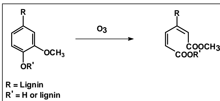
Figure 6 The reaction of lignin with ozone
