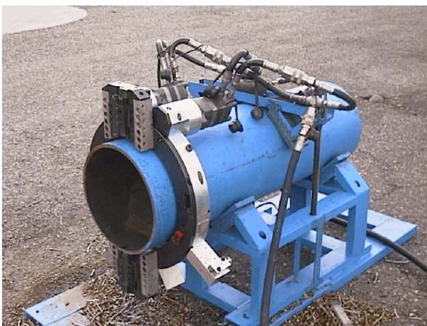
Figure 3. Cutting 61-cm (24-in.) pipe.
