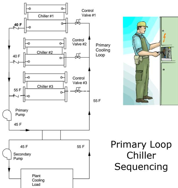
To offset the problem of poor part-load performance, multiple centrifugal chillers may be used in a cooling plant. An optimum chiller sequencing control strategy dispatches the chillers to effectively manage their part-load performance.
