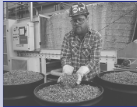
Shredded carpet ready for processing.
