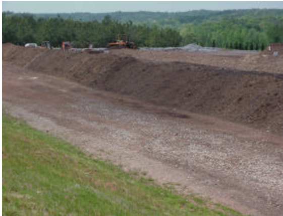
Figure 7. Windrow of yard waste compost with a windrow turner in the background.
