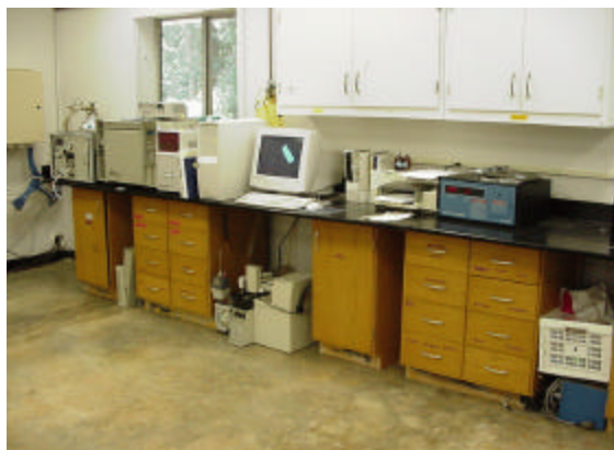
Figure 3. Analysis area photograph showing a gas chromatograph for analyzing off gases from the bench scale composting apparatus
