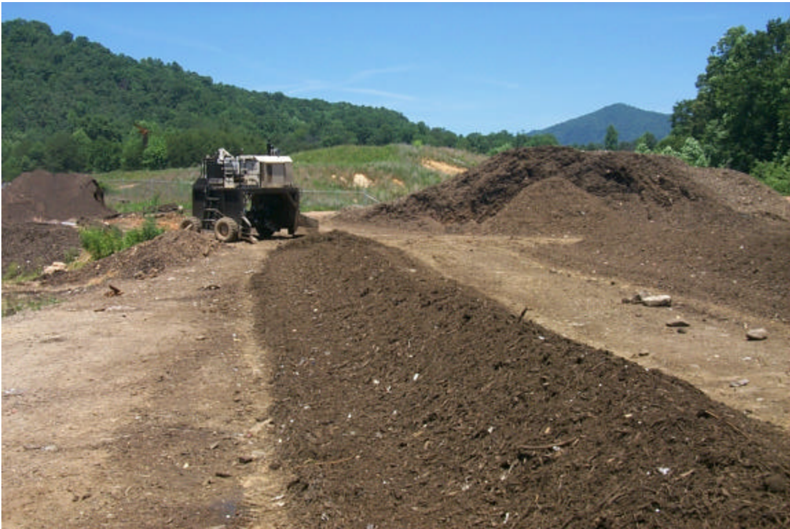
Figure 2 Food Waste Composting Windrows
