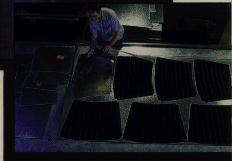
The plasma cutter works on 1 of 2 tables to cut parts to exact specification. The parts layout is very efficient, significantly reducing the scrap rate.
