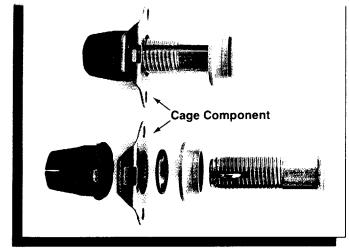
Aerospace fasteners are specifically designed to withstand vibration and remain locked in place. They are corrosion resistant and can withstand an average of 250 cycles of reuse. By using these long-lasting fasteners, an aerospace company can decrease the number of spare parts needed to keep its planes flying.
