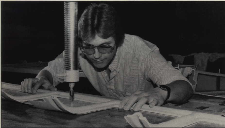
Figure 2. Waterjet cutting composite aircraft parts for the interior cabin eliminates costly trimming and finishing steps.
