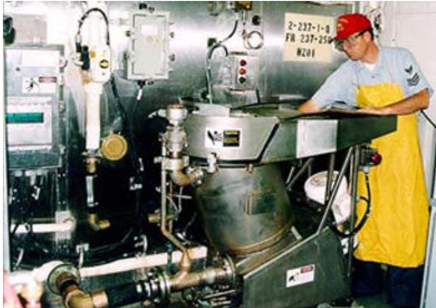
The Small Pulper processes shipboard food, cardboard and paper waste (including classified documents) into a wet slurry for discharge overboard. The Small Pulper is intended for Navy ships that do not have the space available for the Large Pulper, nor require its high processing capability.
