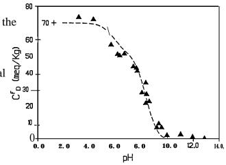
analyze data for the equilibrium **uptake** of C.I. Acid Blue 45 by nylon 6. A good non-linear fit of the experimental data, based on the measured acidic and basic end group contents of the fibers, was obtained from the dimensionless model, as can be seen in the **Figure. The** dimensionless parameters were estimated while fitting the data to the dimensionless model. On
