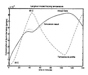
assumed to be driven by two simultaneous processes of adsorption and desorption.
