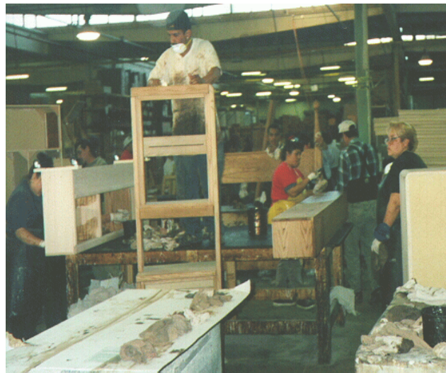
Application of hand-wiped stain
