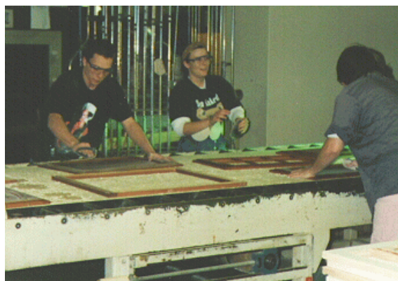
Hand-wiping stain on component edges
