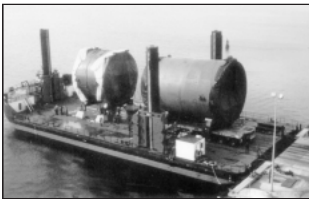
Figure 2-1. Sea Shuttle Jack-Up Barge
