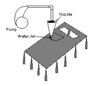
larger nozzles are used. For very hard materials, abrasives may be added to the water to enhance cutting action.
