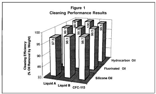
Test conditions: one minute immersion in boiling solvent with sonication followed by one minute vapor rinse.
