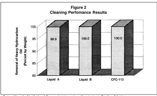
Test conditions for Liquids A and B: one minute immersion with sonication in Petroferm Solvating Agent 24 followed by 30 second immersion rinse in Liquid A or B.
